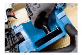
Adjust the plate according to the length of the nails (scale in the magazine.)
