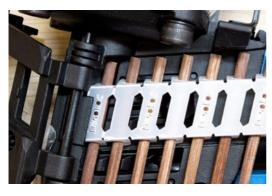
The top of LIGNOLOC® wooden nails must lie flush with the upper edge of the loading channel.
