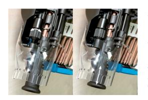
The depth setting can be adjusted by rotating the control wheel located on the front side of the tool.
