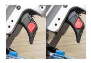
To switch from full sequential actuation to contact actuation: push red button out of the trigger and turn it from front to back position.
